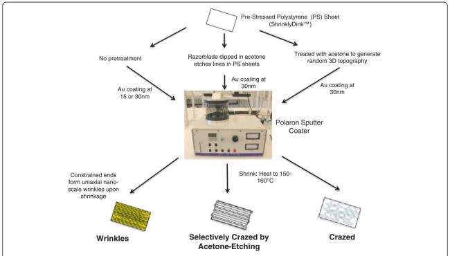
**Figure 1 Microchip Fabrication.** Flowchart of three fabrication methods for the different topographies. The fabrication methods include: two different sizes of **wrinkles** that generate uniaxial nanoscale channels in the molds, selectively crazed **acetone-etched** method that generates larger micron-sized channels, and a **crazed** 'control' topography that does not generate uniform channels, but does exhibit random three-dimensional hills, valleys and ridges.
