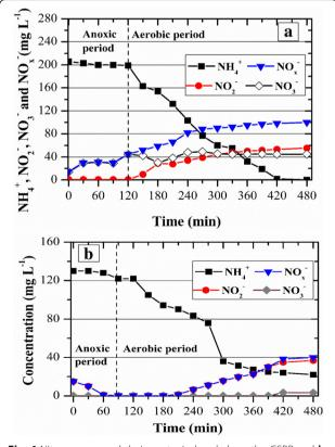
Fig. 4 Nitrogen removal during a typical cycle by  ${\bf a}$  the GSBR and  ${\bf b}$  the ASBR
