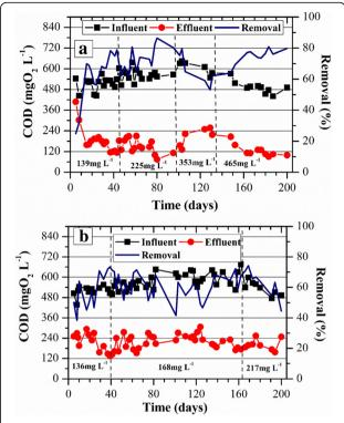
**Fig. 2** COD removal profiles along with time for the aerobic reactors:  $\bf a$  GSBR and  $\bf b$  ASBR. \* The concentrations in the graphs refer to ammonium nitrogen
