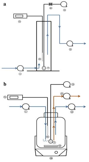
**Fig. 1** Schematic of the **a** GSBR and **b** ASBR: ① feeding pump; ② decanting pump; ③ air compressor; ④ air flow meter; ⑤ pH controller; ⑥ pH meter; ⑦ air diffuser; ⑧ waste sludge pump; ⑨ stir bar; ⑩ magnetic stir plate
