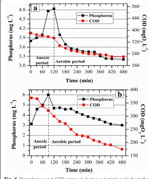
Fig. 6 Phosphorus and COD removal during a typical cycle by  ${\bf a}$  the GSBR and  ${\bf b}$  the ASBR
