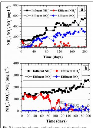
**Fig. 3** Ammonium nitrogen, nitrite nitrogen and nitrate nitrogen profile along with time: **a** GSBR and **b** ASBR
