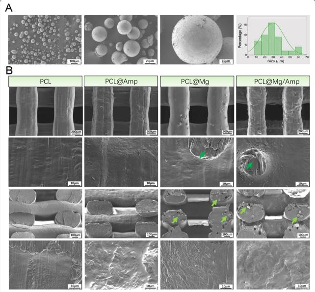
Fig. 2 A SEM images of Mg microparticles and diameter distribution. B SEM images of the surface and cross-section morphology of the scaffold. The green arrow indicates the Mg microsphere
